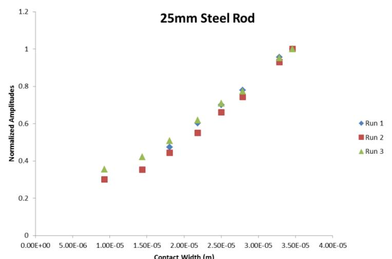
Early results are promising, showing a distinct relationship between reflected amplitudes to contact width. The next step is to theoretically model the physical system to produce a predictive model that would agree with the experimental data.
