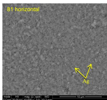
Fig. 2 SEM surface morphology (back-scattered) (21at%Ag)
