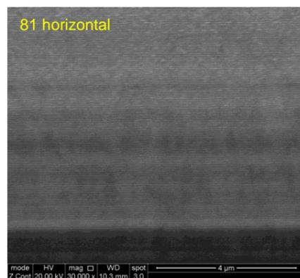
Fig. 1 SEM (back-scattered) image in cross-section (21at%Ag)
