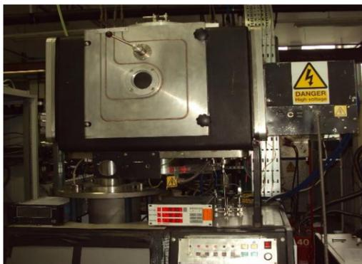
Fig.1 Sputter Deposition Equipment
