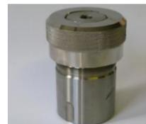
Figure 2: sealed Teflon lined general-purpose bomb
