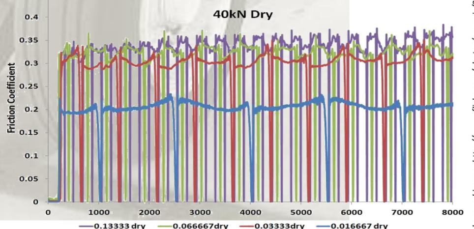
Figure 4 – Friction co efficient for dry contact at 40kN, varying frequencies
