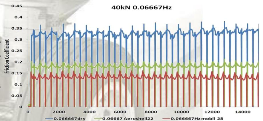
Figure 2 – Friction Coefficients for different lubricants at 40kN, 0.06667 Hz reciprocating Frequency
