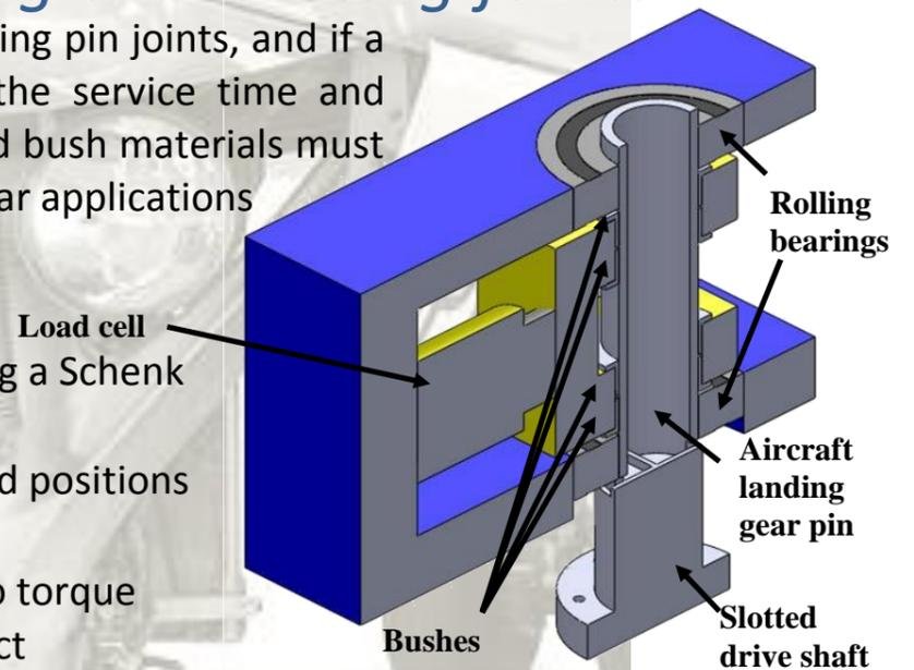
Figure 1 – University of Sheffield pin joint test rig
