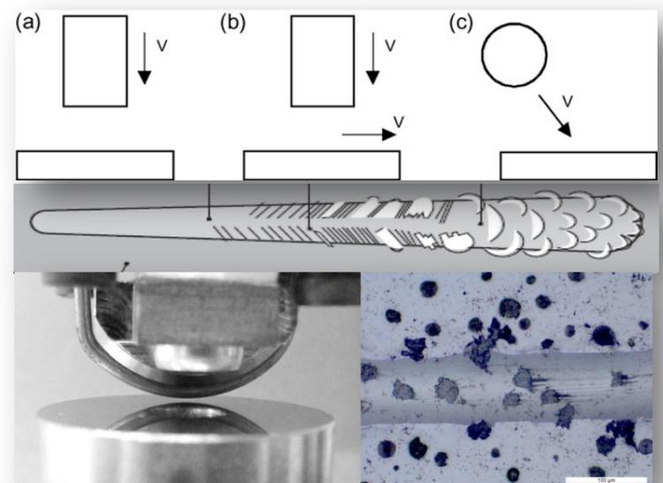
Fig. 2. Down from top: schematic of impact modes (R.Lewis, 2007), typical progressive load failures for DLC coatings, novel steel wire scratch slider (R.Waudby et al, 2012) and scratch track for spherodised cast iron
