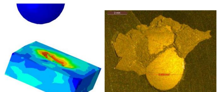
Fig. 3- Peridynamic model of impact event (M.Lindroos, TUT), left, and an impact site from a WC-10Co-4Cr coated sample, right. The impact energy was nearly 55J.
