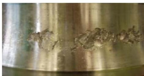
Figure 1: Spalling caused by WSF
