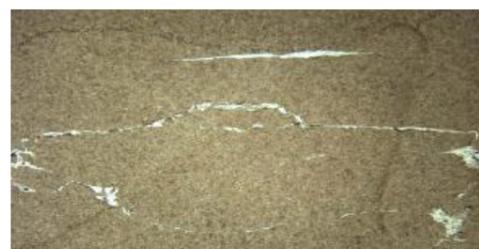
Figure 2: White etching cracks
