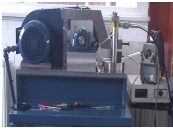
Fig.1 Photo of the bearing test rig
