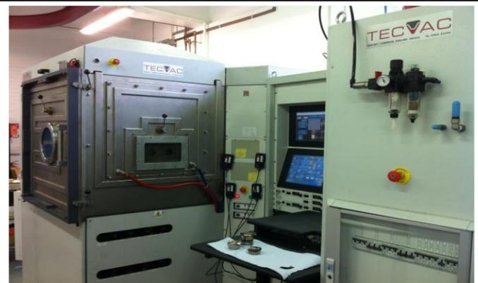
Fig. 1. Magnetron sputtering deposition equipment (TECVAC)
